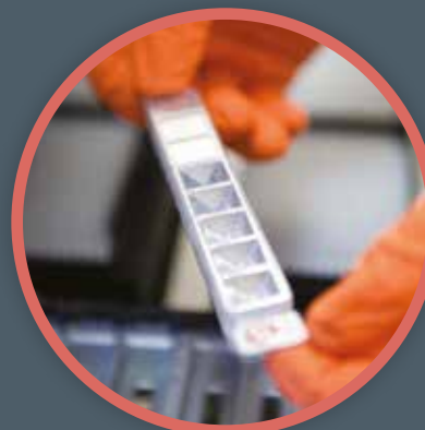
Loading SMRT cell chip strip onto the PacBio RSII sequencing platform.
