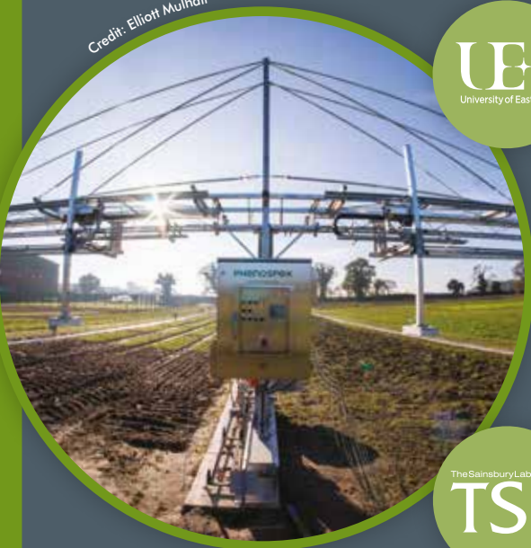
The Phenospex measures growth and development of plants in field conditions.
